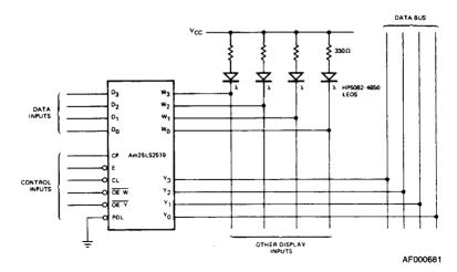
Convenient Register Content Monitor or Test Point
