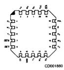
Note: Pin 1 is marked for orientation
