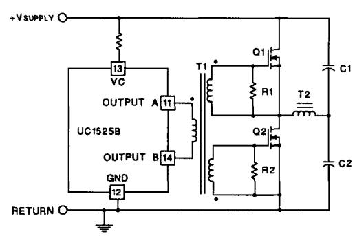
Low power transformers can be driven directly by the UC1525B. Automatic reset occurs during dead time, when both ends of the primary winding are switched to ground.
