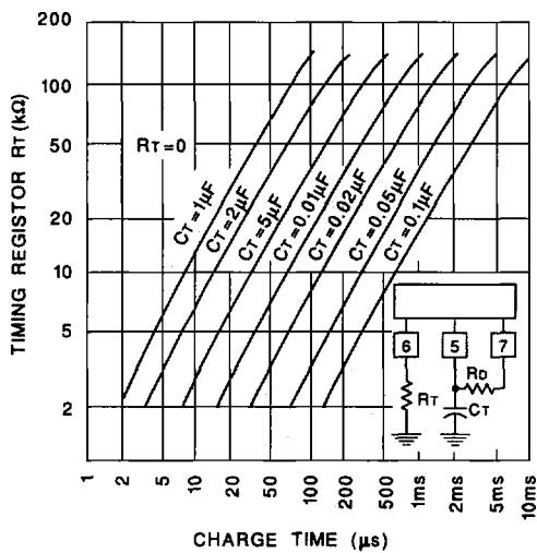
Oscillator Discharge Time vs. R<sub>D</sub> and C<sub>T</sub>
