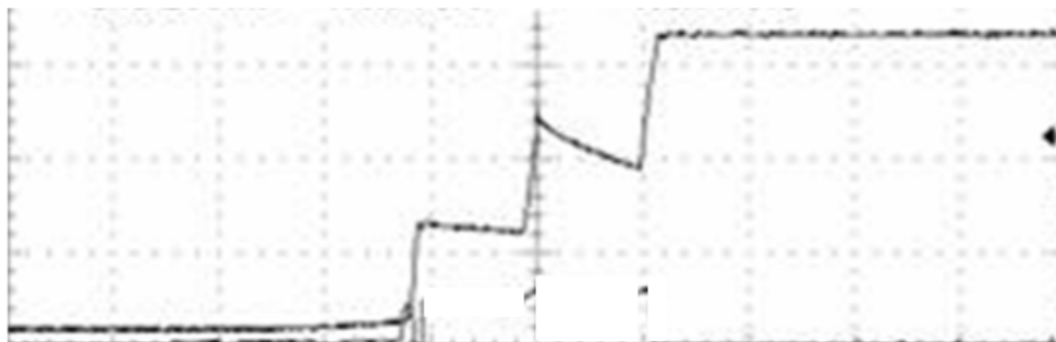
Figure 23. Supply Voltage Drop
