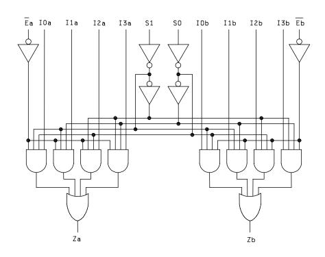
FIGURE 3. Logic diagram.
