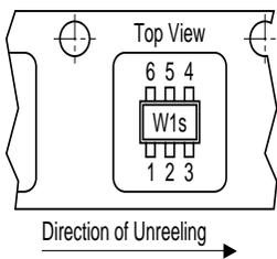
Marking on SOT-363 package (for example W1s) corresponds to pin 1 of device
