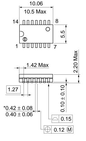
\*Dimension including the plating thickness Base material dimension
