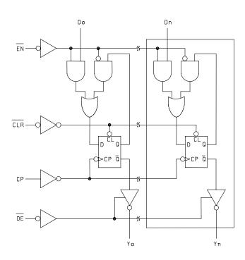
FIGURE 3. Logic diagram.
