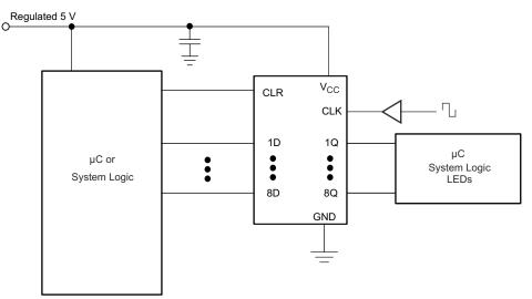
Figure 9-1. Typical Application Schematic
