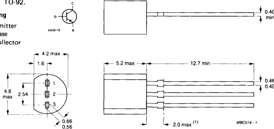
Note (1) Terminal dimensions within this zone are uncontrolled to allow for flow of plastic and terminal irregularities.
