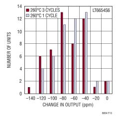
Figure 13. Output Voltage Shift Due to IR Reflow (%)
