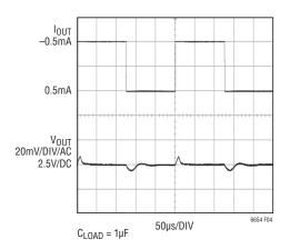
Figure 4. LT6654-2.5 Sourcing and Sinking 0.5mA
