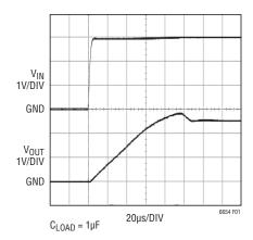
Figure 1. Turn-On Characteristics of LT6654-2.5
