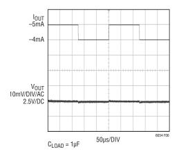
Figure 6. LT6654-2.5 Sinking 4mA to 5mA
