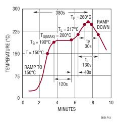
Figure 12. Lead Free Reflow Profile
