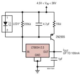
\*LED CANNOT BE OMMITTED THE LED CLAMPS THE VOLTAGE DROP ACROSS THE  $220\Omega$  AND LIMITS OUTPUT CURRENT
