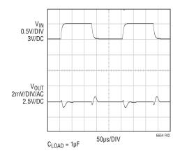
Figure 2. Output Response to 0.5V Ripple on V<sub>IN</sub>
