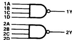
$$\text{positive logic } Y = \overline{A \cdot B \cdot C \cdot D} \text{ or } Y = \overline{A} + \overline{B} + \overline{C} + \overline{D}$$
