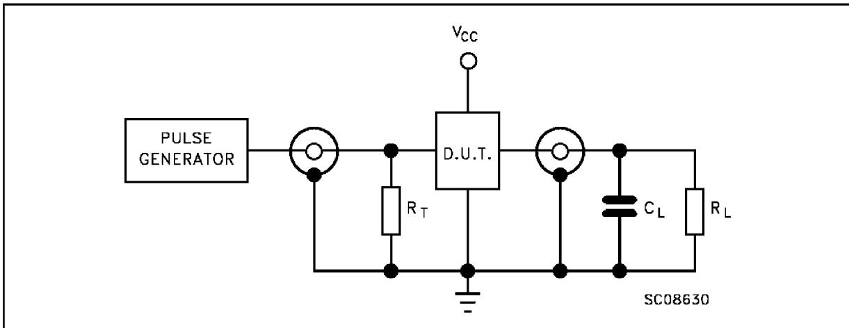
$C_L = 50 \text{ pF}$  or equivalent (includes jig and probe capacitance)
