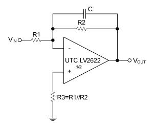
Figure 6. Low Pass Active Filter
