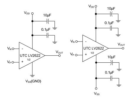
Figure 3. Amplifier with Bypass Capacitors
