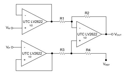
Figure 5. Instrumentation Amplifier
