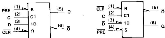
Notice that Q and  $\bar{Q}$  exchange names, which causes Preset and Clear to do likewise. Also notice that the polarity indicators (Δ) on  $\overline{\text{PRE}}$  and  $\overline{\text{CLR}}$  remain since these inputs are still active-low, but that the presence or absence of the polarity indicator changes at  $\overline{D}$ , Q, and  $\bar{Q}$ . Of course pin 5 ( $\bar{Q}$ ) is still in phase with the data input  $\overline{D}$ , but now both are considered active-low.
