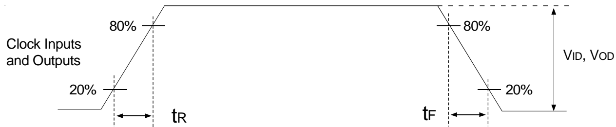
Figure 8. Input and Output Slew Rates
