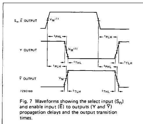
Fig. 7 Waveforms showing the select input ( $S_n$ ) and enable input ( $\bar{E}$ ) to outputs ( $Y$  and  $\bar{Y}$ ) propagation delays and the output transition times.
