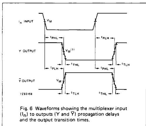
Fig. 6 Waveforms showing the multiplexer input ( $I_n$ ) to outputs ( $Y$  and  $\bar{Y}$ ) propagation delays and the output transition times.
