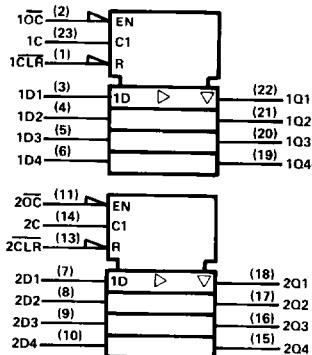
functional block diagram (each quad latch, positive logic)
