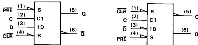
Notice that Q and  $\bar{Q}$  exchange names, which causes Preset and Clear to do likewise. Also notice that the polarity indicators ( $\downarrow$ s) on PRE and CLR remain since these inputs are still active-low, but that the presence or absence of the polarity indicator changes at  $\bar{D}$ , Q, and  $\bar{Q}$ . Of course pin 5 ( $\bar{Q}$ ) is still in phase with the data input  $\bar{D}$ , but now both are considered active-low.
