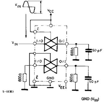
**BANDWIDTH AND FEEDTHROUGH ATTENUATION**
