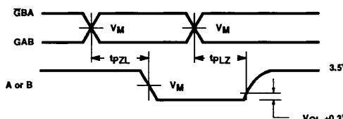
Waveform 4. 3-State Output Enable Time to Low Level Output Disable Time from Low Level
