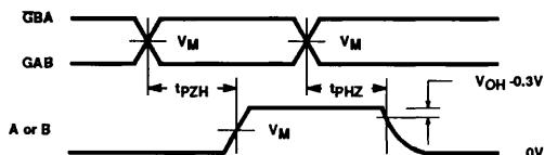
Waveform 3. 3-State Output Enable Time to High Level Output Disable Time from High Level
