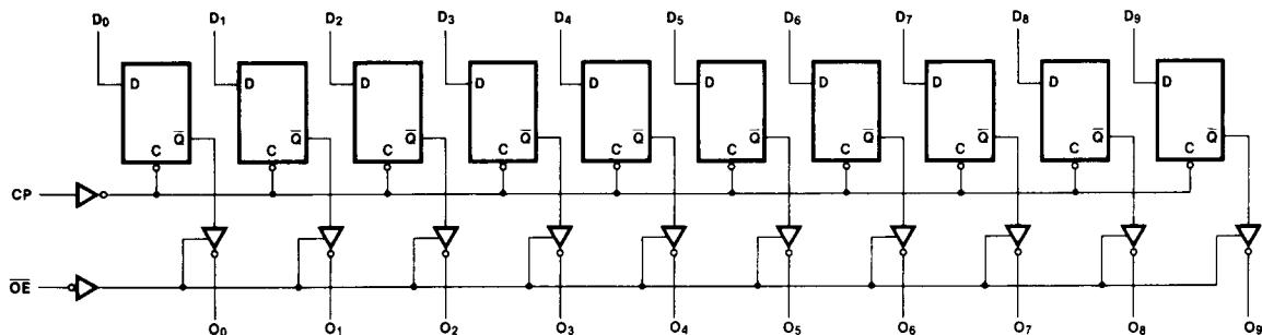
Please note that this diagram is provided only for the understanding of logic operations and should not be used to estimate propagation delays. The 'AC/'ACT822 also has the same logic diagram with inverting outputs.
