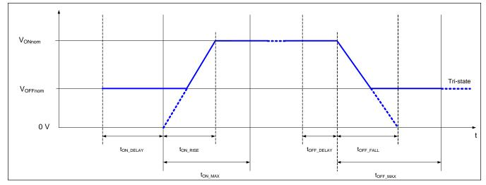
Figure 3.2 Power Sequencing with Non-zero Off Voltage
