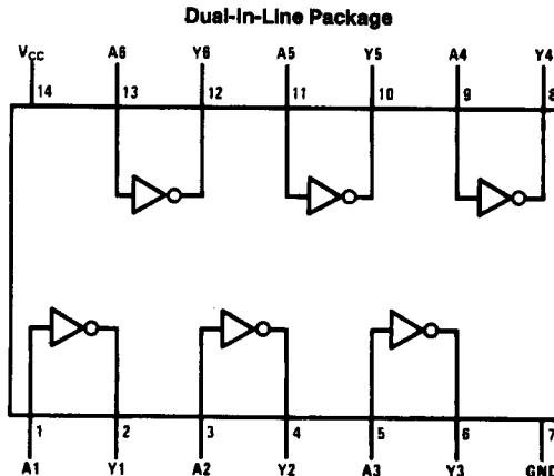
Order Number 54LS04DMQB, 54LS04FMQB, 54LS04LMQB, DM54LS04J, DM54LS04W, DM74LS04M or DM74LS04N
