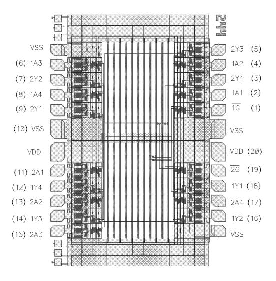
Note: Pad numbers reflect terminal numbers when placed in Case Outlines R and X see figure 1.
