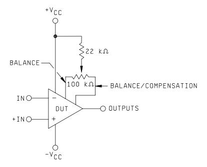
FIGURE 2. Offset null circuit.
