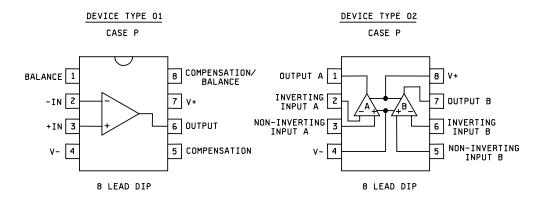
Figure 1. Terminal connections and logic diagram.
