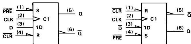
Notice that Q and  $\bar{Q}$  exchange names, which causes Preset and Clear to do likewise. Also notice that the polarity indicators ( $\Delta$ ) on PRE and  $\overline{\text{CLR}}$  remain since these inputs are still active-low, but that the presence or absence of the polarity indicator changes at  $\bar{D}$ , Q, and  $\bar{Q}$ . Of course pin 5 ( $\bar{Q}$ ) is still in phase with the data input  $\bar{D}$ , but now both are considered active-low.
