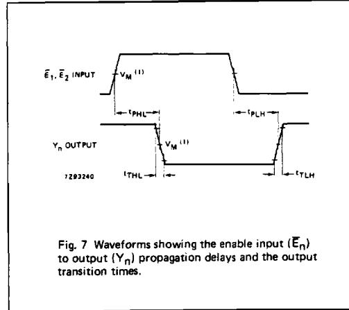
Fig. 7 Waveforms showing the enable input ( $E_n$ ) to output ( $Y_n$ ) propagation delays and the output transition times.
