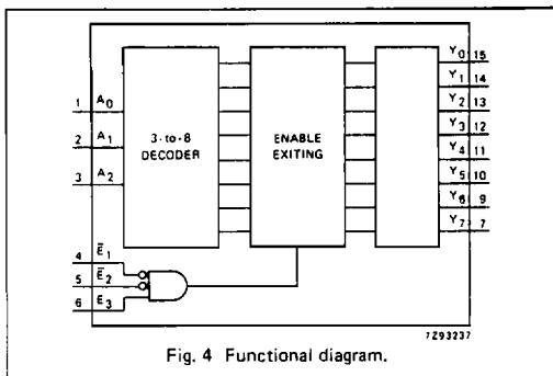
Fig. 4 Functional diagram.
