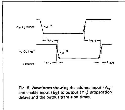
Fig. 6 Waveforms showing the address input ( $A_n$ ) and enable input ( $E_3$ ) to output ( $Y_n$ ) propagation delays and the output transition times.
