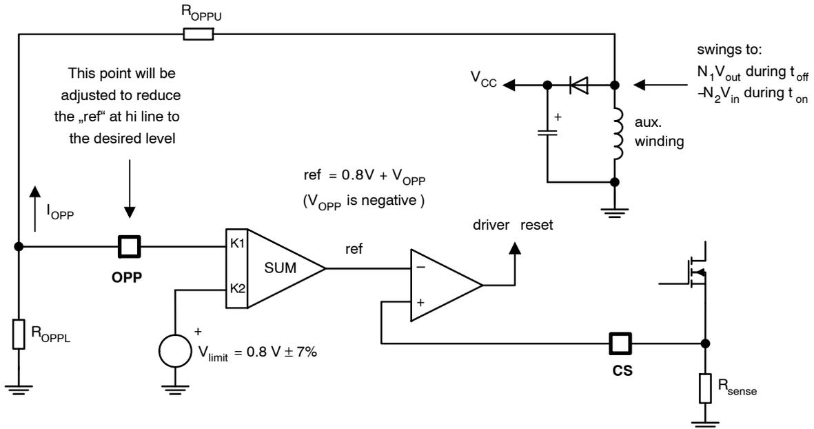
Figure 34. The OPP Circuitry Affects the Maximum Peak Current Set Point by Summing a Negative Voltage to the Internal Voltage Reference
