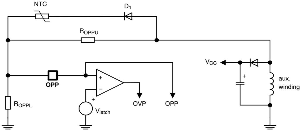
**Figure 40. The Internal Circuitry Hooked to OPP Pin can be used to Implement Over Temperature Protection (OTP)**
