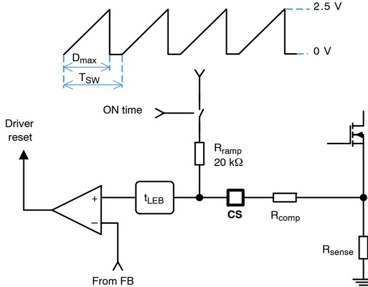
**Figure 36. Inserting a Resistor in Series with the Current Sense Information Brings Slope Compensation and Stabilizes the Converter in CCM Operation**
