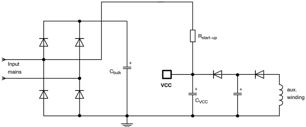
Figure 32. The Startup Resistor can be Connected to the Input Mains for further Power Dissipation Reduction
