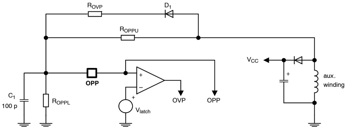
**Figure 38. A Simple Resistive Divider Brings the OPP Pin above 3 V in case of a  $V_{CC}$  Voltage Runaway above 18 V**
