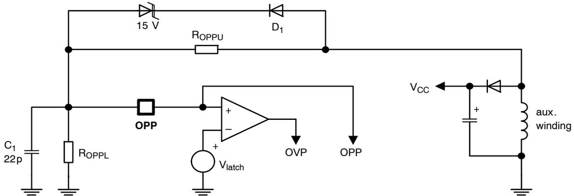
Figure 39. A Zener Diode in Series with a Diode Helps to Improve the Noise Immunity of the System
