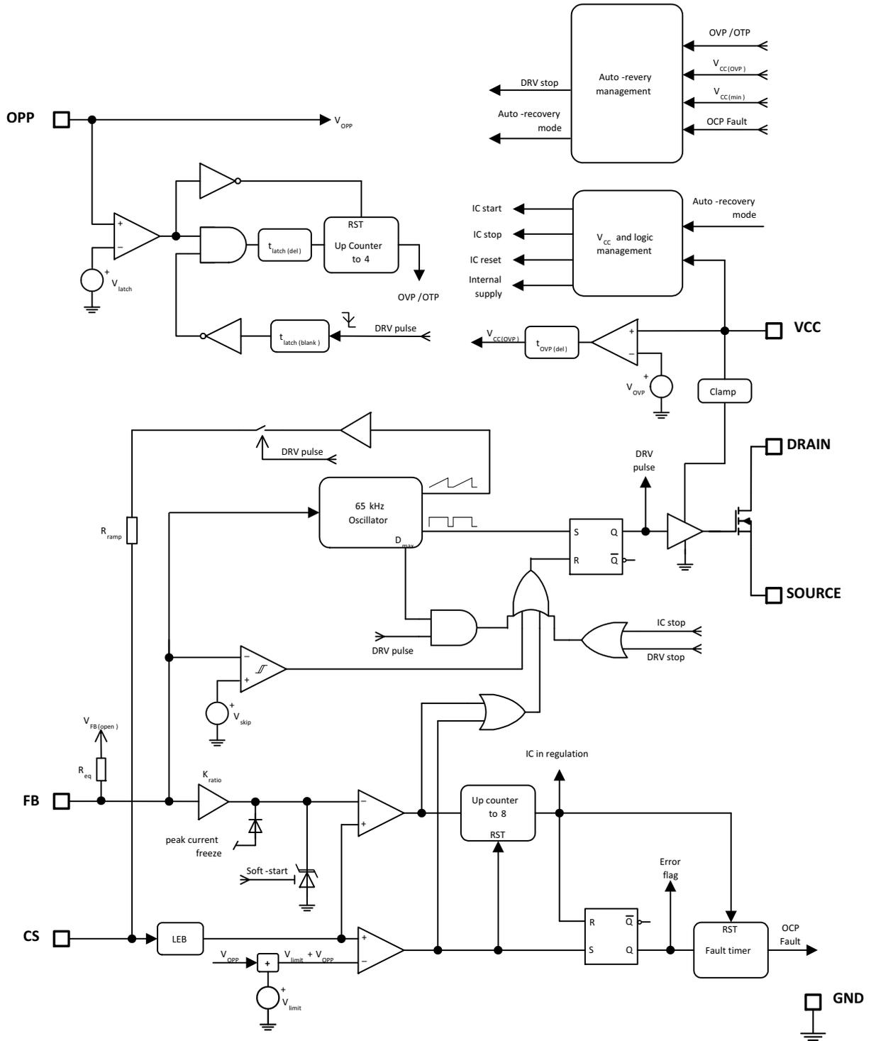
Figure 3. Internal Circuit Architecture
