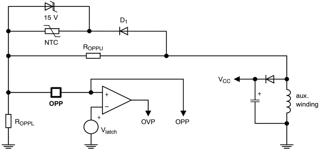
**Figure 41. With the NTC Back in Place, the Circuit Nicely Combines OVP, OTP and OPP on the Same Pin**
