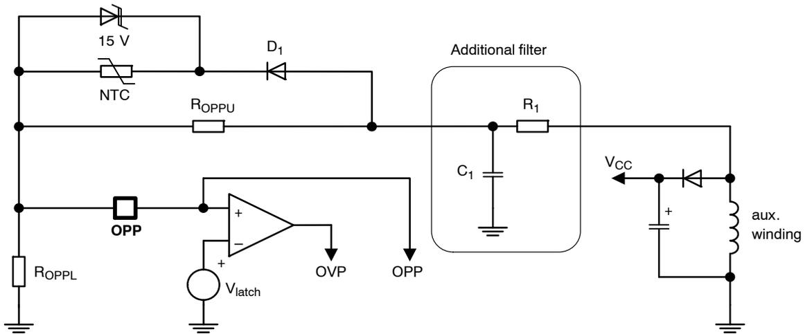
**Figure 42. A Small RC Filter Prevents the Fast Rising Spikes from Reaching the Protection Pin OPP in Presence of Energetic Perturbations Superimposed on the Input Line**
