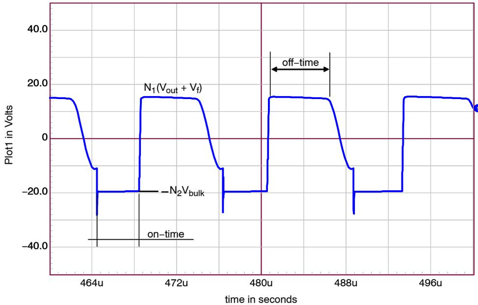
Figure 33. The Signal Obtained on the Auxiliary Winding Swings Negative During the On-time
