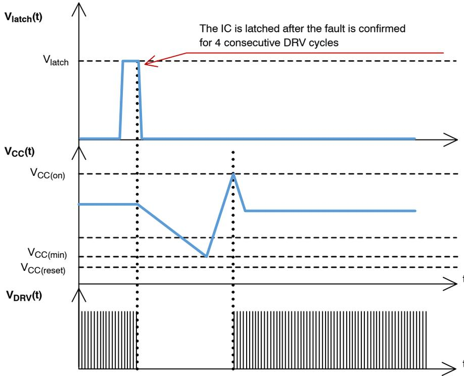
**Figure 37. Auto-recovery of the Controller and Resuming Operation**
