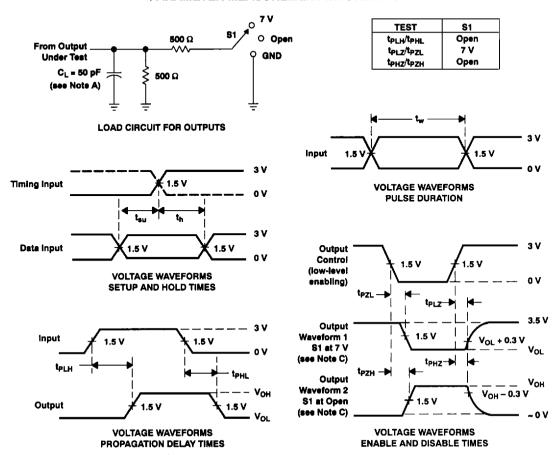
NOTES: A. Ct includes probe and jig capacitance.
