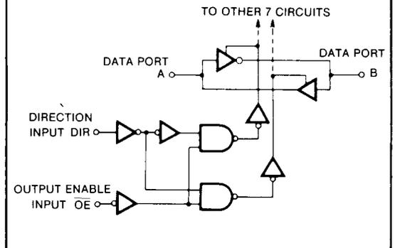
**OCTAL 3-STATE INVERTING AND NONINVERTING BUS TRANSCEIVER**
