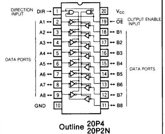
**LOGIC DIAGRAM (EACH TRANSCEIVER)**
