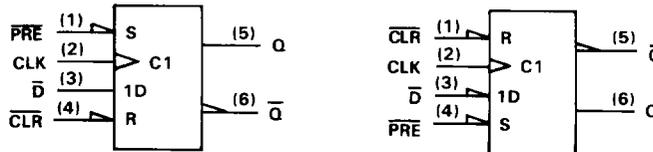
Notice that Q and  $\bar{Q}$  exchange names, which causes Preset and Clear to do likewise. Also notice that the polarity indicators ( $\bar{\square}$ ) on PRE and CLR remain since these inputs are still active-low, but that the presence or absence of the polarity indicator changes at  $\bar{D}$ , Q, and  $\bar{Q}$ . Of course pin 5 ( $\bar{Q}$ ) is still in phase with the data input  $\bar{D}$ , but now both are considered active-low.
