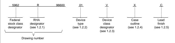
1.2.1 <u>RHA designator</u>. Device class M RHA marked devices shall meet the MIL-I-38535 appendix A specified RHA levels and shall be marked with the appropriate RHA designator. Device classes Q and V RHA marked devices shall meet the MIL-I-38535 specified RHA levels and shall be marked with the appropriate RHA designator. A dash (-) indicates a non-RHA device.
