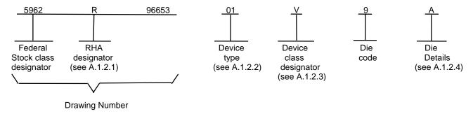
A.1.2.1 <u>RHA designator</u>. Device classes Q and V RHA identified die shall meet the MIL-PRF-38535 specified RHA levels. A dash (-) indicates a non-RHA die.
