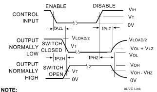
1. Diagram shown for input Control Enable-LOW and input Control Disable-HIGH.
