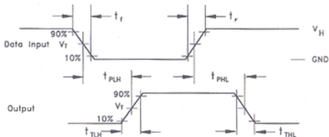
Input and Output Threshold Voltage: V<sub>T</sub> = 50% V<sub>CC</sub> for HC, 1.3V for HCT, V<sub>H</sub> = V<sub>CC</sub> for HC, 3V for HCT
