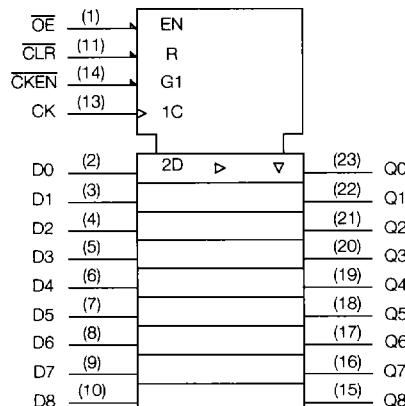
The TC74ACT823 is an advanced high speed CMOS 9-BIT BUS D-TYPE FLIP-FLOP with 3-STATE OUTPUT fabricated with silicon gate and double-layer metal wiring C<sup>2</sup>MOS technology.
