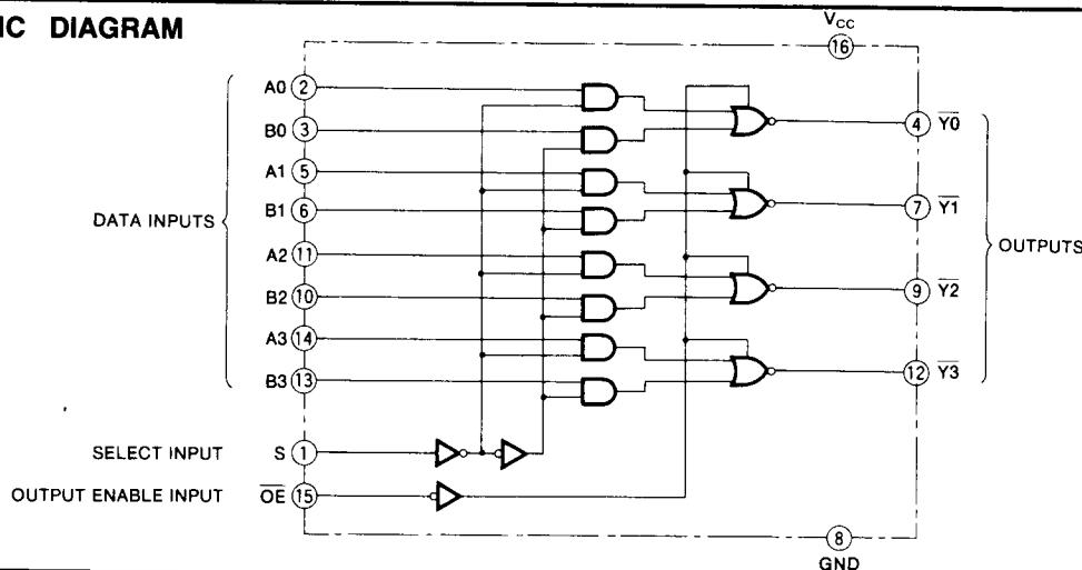
QUADRUPLE 2-INPUT DATA SELECTOR/MUX WITH 3-STATE OUTPUTS
