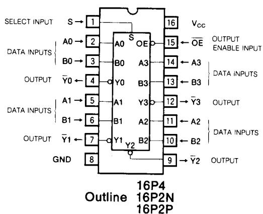
at  $\bar{Y}$  in synchronous with the clock pulse in the order A-B. S and output-enable input  $\bar{OE}$  are common to all four circuits. When  $\bar{OE}$  is high, all outputs Y will become high impedance state irrespective of other inputs.
