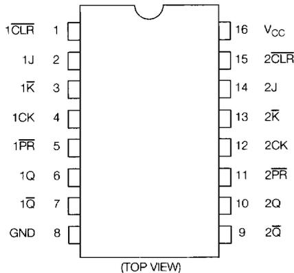
The TC74ACT109 is an advanced high speed CMOS DUAL J-K̄ FLIP-FLOP fabricated with silicon gate and double-layer metal wiring C<sup>2</sup>MOS technology.
