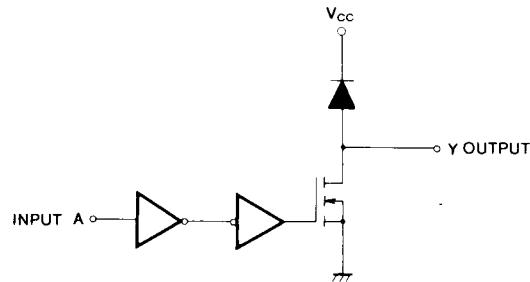
HEX INVERTER WITH OPEN-DRAIN OUTPUTS
