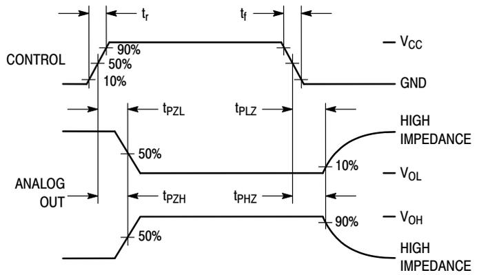
**Figure 10. Propagation Delay, ON/OFF Control to Analog Out**
