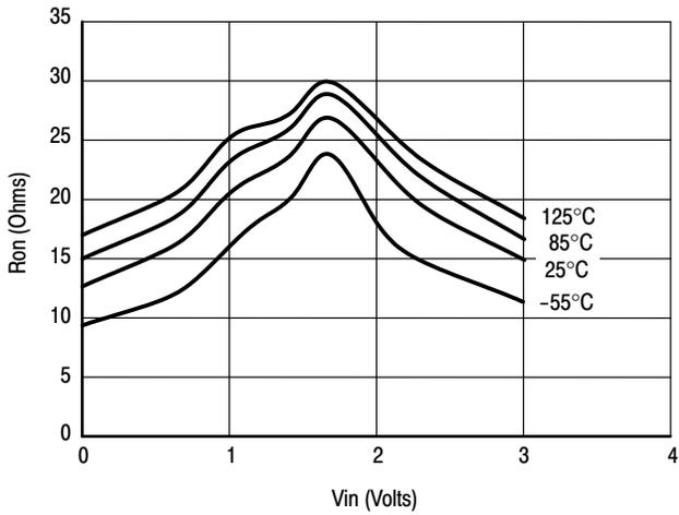
Figure 1c. Typical On Resistance,  $V_{CC} = 3.0\text{ V}$
