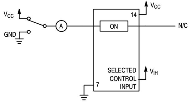
Figure 4. Maximum On Channel Leakage Current, Test Set-Up
