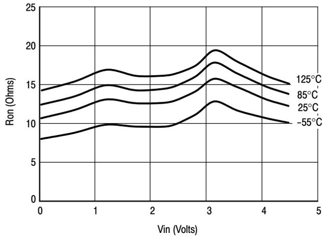
Figure 1d. Typical On Resistance,  $V_{CC} = 4.5\text{ V}$
