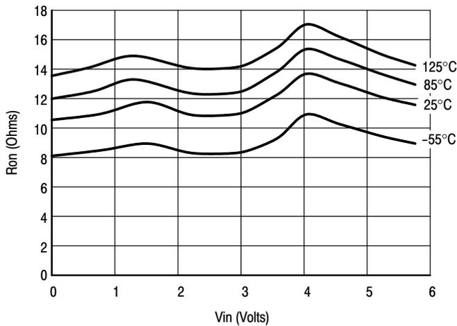
Figure 1e. Typical On Resistance,  $V_{CC} = 5.5\text{ V}$
