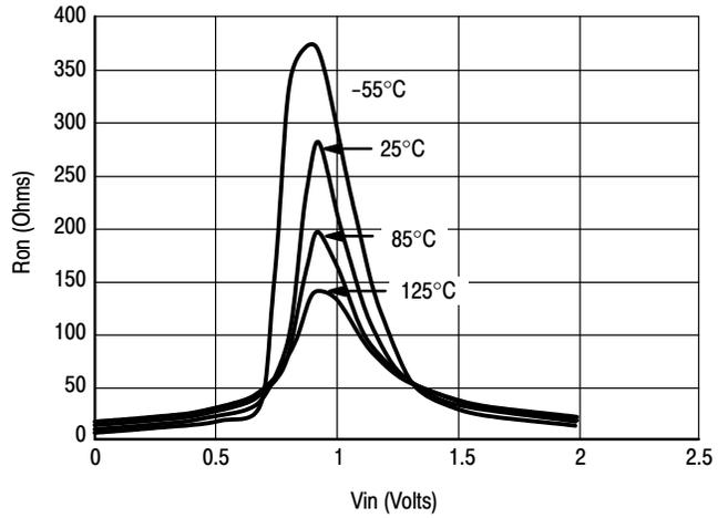
Figure 1b. Typical On Resistance,  $V_{CC} = 2.0\text{ V}$
