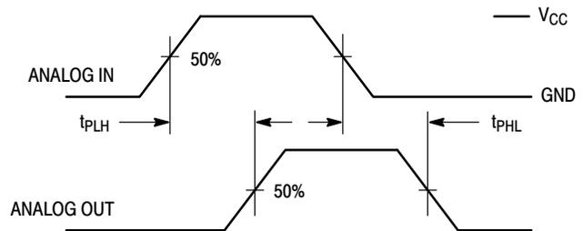
Figure 8. Propagation Delays, Analog In to Analog Out
