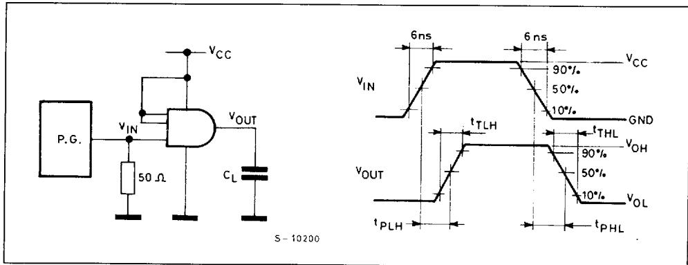
TEST CIRCUIT I<sub>CC</sub> (Opr.)
