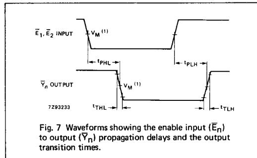
Fig. 7 Waveforms showing the enable input ( $\bar{E}_n$ ) to output ( $\bar{Y}_n$ ) propagation delays and the output transition times.
