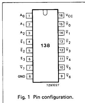
Fig. 1 Pin configuration.
