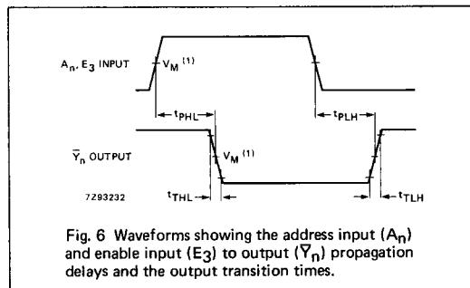
Fig. 6 Waveforms showing the address input ( $A_n$ ) and enable input ( $E_3$ ) to output ( $\bar{Y}_n$ ) propagation delays and the output transition times.
