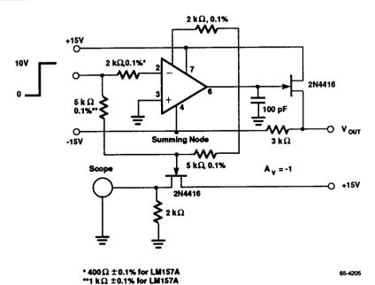
Settling -Time Test Circuit
