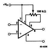
Note: For potentiometers with a temperature coefficient < 100 ppm/  $^{\circ}$ C, the added TCV<sub>08</sub> with nulling is  $\approx 0.5 \mu V/^{\circ}$ C /mV of adjustment
