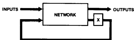
Figure 5b. The feedback of figure 5a is broken to convert the system to a non-sequential one
