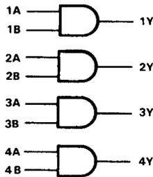
$$Y = A \cdot B \text{ or } Y = \overline{\overline{A} + \overline{B}}$$
