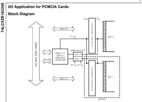
The LCXZR163245 is a 48-pin dual supply device well suited for PCMCIA I/O applications. Ideal for low power notebook designs, the LCXZR163245 consumes less than 1 mW of quiescent power in all modes of operation. The LCXZR163245 meets all PCMCIA I/O voltage requirements at 5V and 3.3V operation. By tying V<sub>CCB</sub> of the LCXZR163245 to the card voltage supply, the PCMCIA card will always experience rail to rail output swings, maximizing the reliability of the interface.
