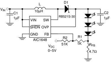
Fig. 18 Dimming Control Using a DC Voltage
