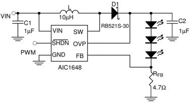
Fig. 16 Dimming Control with a PWM Signal
