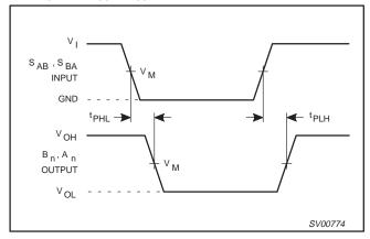
Figure 3. Input S<sub>AB</sub>, S<sub>BA</sub> to output B<sub>n</sub>, A<sub>n</sub> propagation delay times.
