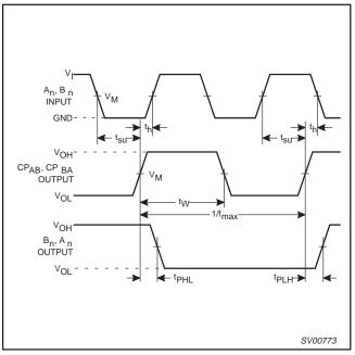
Figure 2.  $\,A_n,\,B_n$  to  $CP_{AB},\,CP_{BA}$  set-up and hold times, clock CP<sub>AB</sub>, CP<sub>BA</sub> pulse width, maximum clock pulse frequency and the  $CP_{AB}$ ,  $CP_{BA}$  to output  $B_n$ ,  $A_n$  propagation delays.
