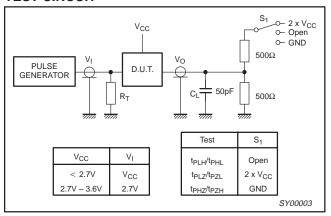
Figure 5. Load circuitry for switching times.
