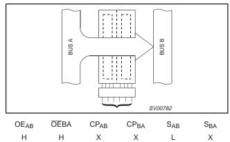
Transfer A stored data to B bus or B stored data to A bus or both at the same time
