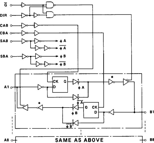
Note: In case of TC74AC646 output inverter marked \* at A bus and B bus are eliminated.
