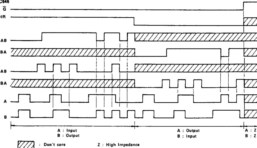
Note: The timing chart for TC74AC648 is the same, but with the outputs inverted.
