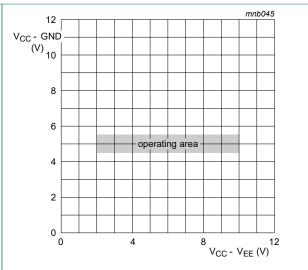
Fig. 5. Guaranteed operating area as a function of the supply voltages for 74HC4052-Q100
