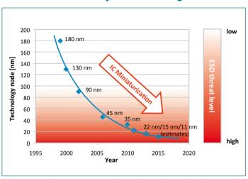
The ultra-small process technologies used to produce today's miniature semiconductors have the side-effect of making the ICs more vulnerable to voltage transients caused by ESD strikes. NXP's PESD5V0X1U family supports these highly sensitive ICs by providing high-performance ESD protection.
